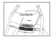
Hold the contacts for approximately ten seconds. When your pulse is detected, your heart rate will be shown. For the most accurate heart rate reading, continue to hold the contacts for about 15 seconds.
